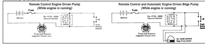
**REMOTE CONTROL:** Install a pushbutton switch at one or more locations (multiple switches should be wired parallel). Depress pushbutton for 2 seconds. If there is water in bilge, pump will operate until dry, at which time vacuum switch will stop pump. If no water is in bilge, pump will stop when pushbutton is released.
